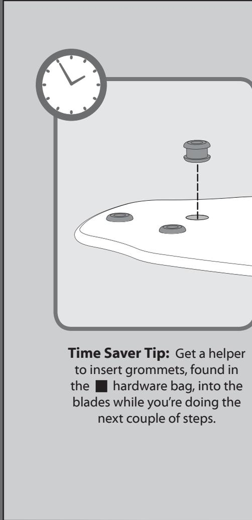
**Time Saver Tip:** Get a helper to insert grommets, found in the ■ hardware bag, into the blades while you're doing the next couple of steps.
