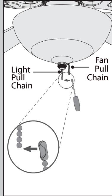
Connect the appropriate pull chain pendant to each of the short chains coming from the finial cap and finial. The fan pull chain controls the speed: from high to off. The light pull chain controls the light fixture: on and off.
