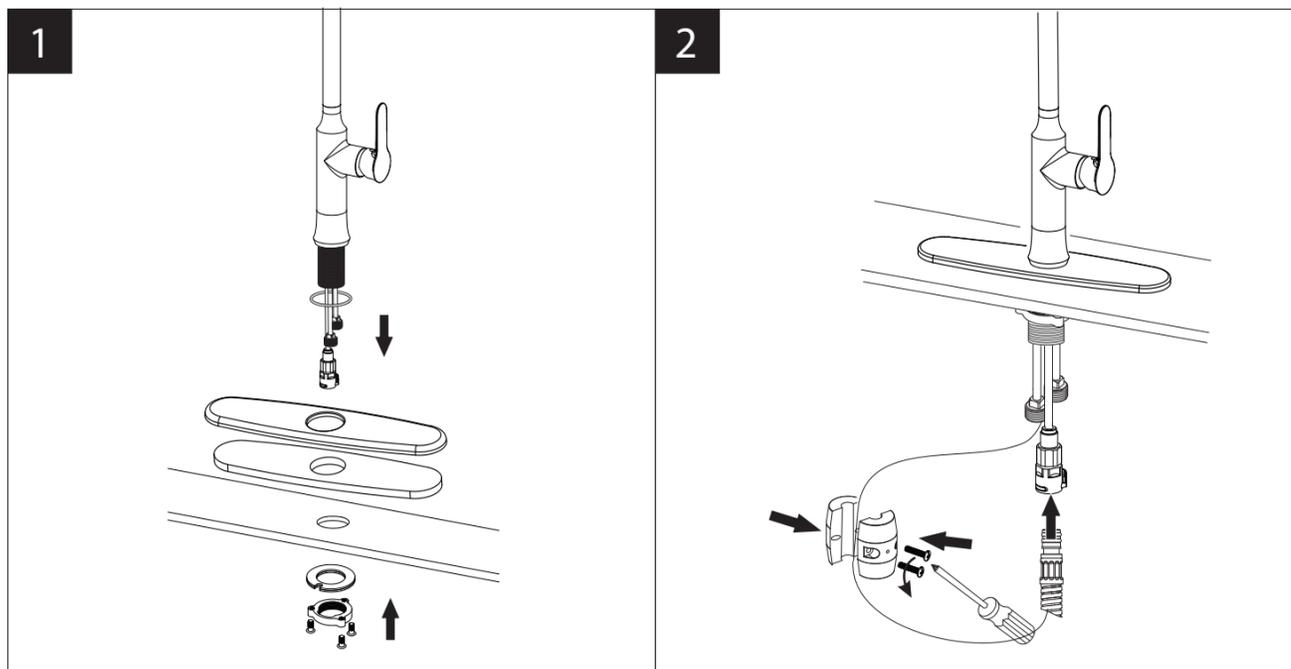
1. Position the faucet, deck plate and gasket in order on the counter top as shown. Don't forget the O-ring. Assemble gasket assembly and lock nut to faucet threaded sleeve by hand and tighten the screws with screwdriver.
