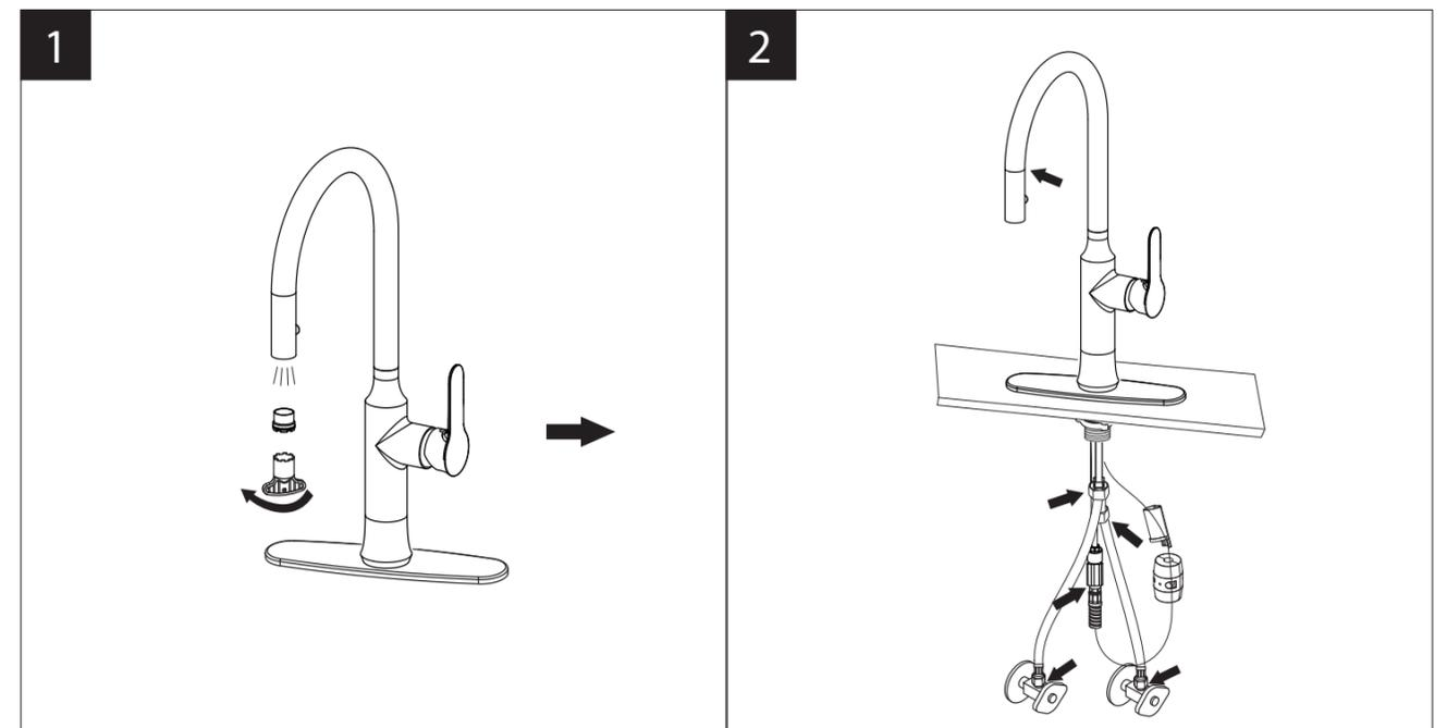
1. Remove the shower by aerator wrench. Turn the faucet handle all the way on, turn on hot and cold water supply and flush water lines for one minute. Reinstall shower by aerator wrench.
