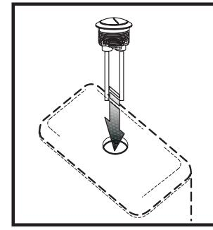
Cut the rod to a proper length, put the push button into the hole.
