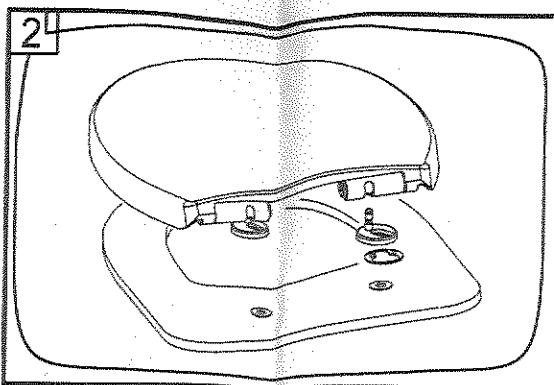
Mount the hinges onto the shaft of the toilet seats.
