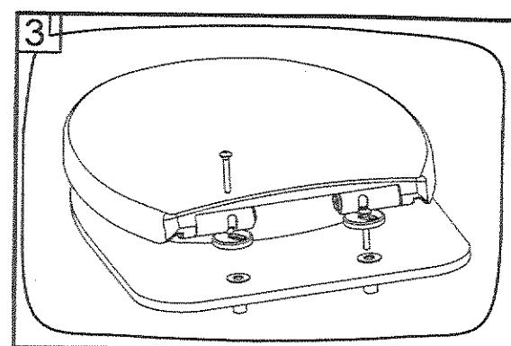
Plug the bolt into the expansion rubber.
