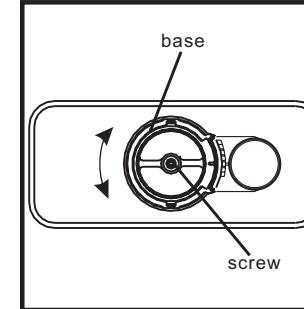
Install the flush valve base into the outlet to make the "U" clasp can clip on the tank properly. Rotate the base to choose proper angleand lock the screw.
