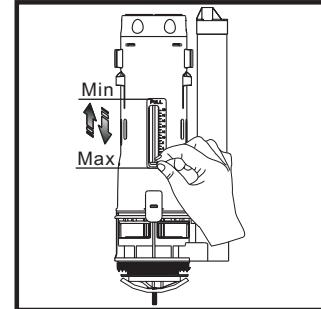
Adjustment of whole flush level: when the white card is on the highest position, the whole flush water is at the least.
