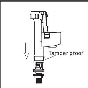
After adjusting height of Fill valve, rotate the upper shank counter clockwise to unlock into lower shank. Next, push down on Tamper proof to secure it.
