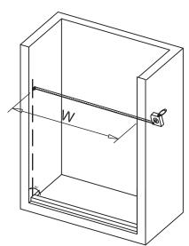
2. Your Upper Guide Rail [5] and Bottom Guide Rail [10] have been precut for your Shower model opening width, eg.60" for shower width. If W-width of your wall-to-wall opening is equal to the size of your Shower model, it is unnecessary to cut the Upper Guide Rail and Bottom Guide Rail and you can continue to Step 3.
