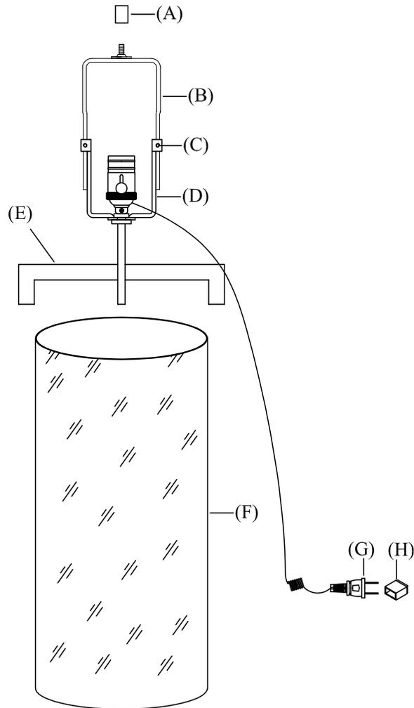
1. Carefully place the cross part assembly (E) on glass cylinder (F). Note: if one side of glass cylinder DOES NOT fit in cross part (B), DO NOT TRY TO FORCE IT. Please turn it over, try to fit another side in.
