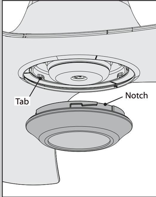
Position the notches in the outer rim of the glass lens cap so they line up with the tabs on the inside of the rim on the LED assembly.
