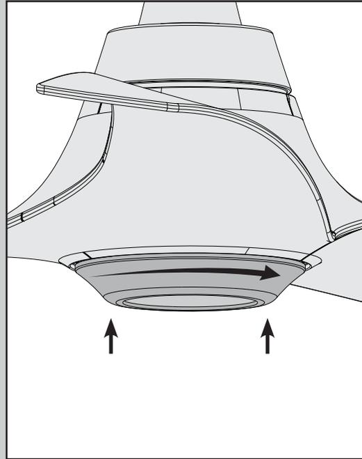
Carefully lift the glass lens cap up inside the LED assembly as far as it will go, then rotate the cap clockwise until it is held tightly in place by the tabs.
