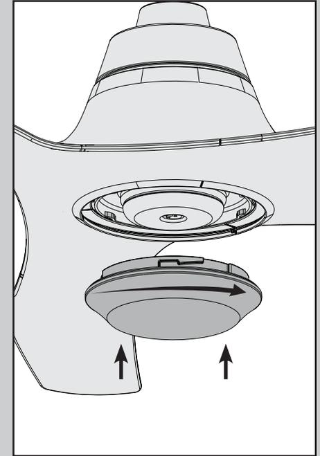
Carefully lift the no-light cap up inside the LED assembly as far as it will go and rotate the cap clockwise until it is held tightly in place by the tabs.
