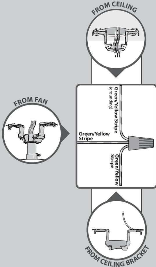
Using an orange wire connector from the ★ hardware bag, connect the three grounding wires (green, green/yellow stripe, or bare copper) coming from the ceiling, downrod, and hanging bracket.
