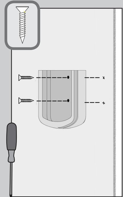
⊗ To install the transmitter cradle, hand-tighten the provided screws to mount the cradle to the wall.
