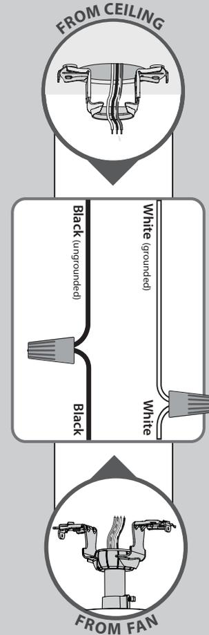
Using orange wire connectors from the ★ hardware bag, connect the black wire (ungrounded) from the ceiling to the black wire from the fan. Connect the white wire (grounded) from the ceiling to the white wire from the fan.
