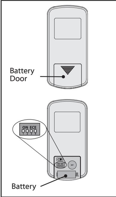
Remove the battery door. Change the DIP switch settings if the frequency matches a previously installed remote transmitter. Install an A23 or MN21 alkaline battery.
