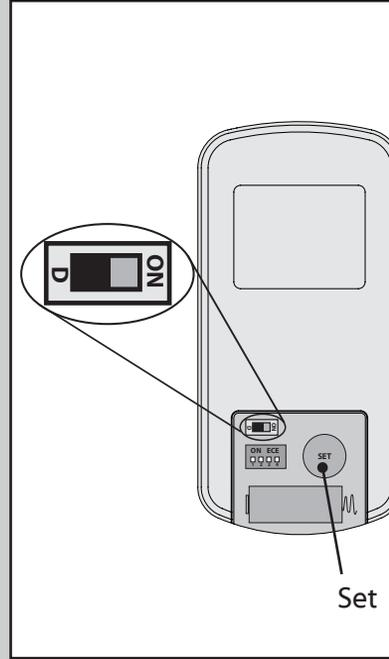
**To pair the remote, hold down the Set button for 5 seconds.** Pairing is complete when the LED button flashes twice. Move the toggle switch to “D” for full-range light dimming or “ON” for on/off function only.
