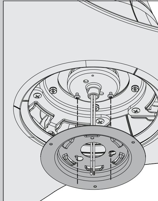
Feed the two single-pin connectors through the center hole of the upper switch housing, then wrap the keyhole slots around the screws and twist counterclockwise.
