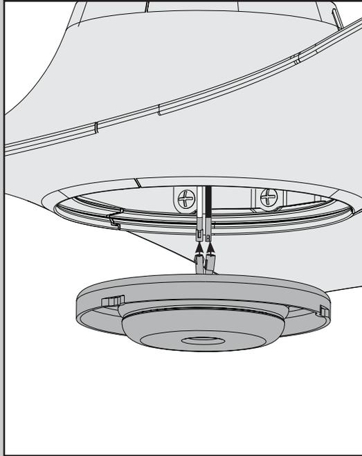
Connect the single-pin connectors from the LED assembly to the connectors from the fan.
