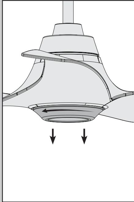
Carefully rotate the glass lens cap counterclockwise until it comes loose from the tabs and lower it from inside the LED assembly.
