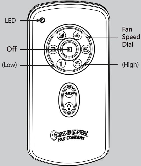
To select a fan speed press one of the numbers on the Fan Speed Dial. To calibrate the fan speed, run the fan on "6" for 90 seconds after each AC power reset. The LED light flashes to indicate a signal has been sent to the fan.
