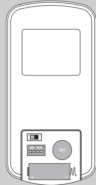
To change the battery, remove the battery door. Remove the battery and replace it with an A23 or MN21 alkaline battery.
