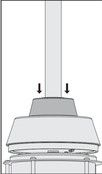
Lower the adapter cover until it rests flush against the motor housing.
