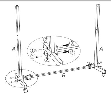
Assemble buttom part of support. Make sure the casters are on the same side.
