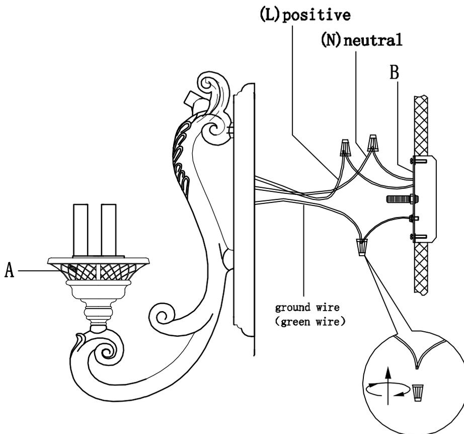
2. Caulk around backplate where fixture meets the wall leave a hole at the bottom to allow water to escape.
