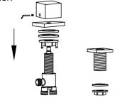
4. Fixed the switch and fasten the nut. Fix the converter handle by the hexagonal tool.
