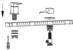
6. Pulling pipe connect with the conversion A through the shower holder. Gravity ball fixed on the top of the pull out pipe. Water nozzle connect to he conversion B, switch water outlet connect to the connector C and
