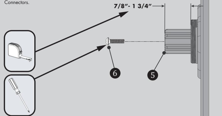
**5** Place Wall Plate (3) onto Mounting Base. Verify the Diverter Valve Stem is in the OFF (vertical) position. Align the Diverter Drive Tube (4) on the Wall Plate to the Stem (5) of the Diverter Valve. Handle shown for reference only.
