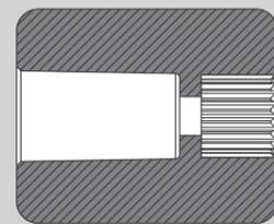
**3** Confirm that the valve is in the "OFF" position. Place appropriate Connector (5) onto spindle of valve making sure to orient the Connector so that one set of splines are perfectly vertical as shown below.
