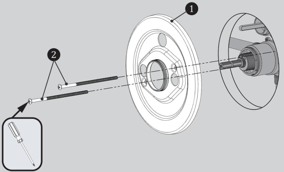
**2** There are two connectors included to allow for both Shallow Mount or Deep Mount applications from finished wall surface. Please select Connector appropriate for your installation.
