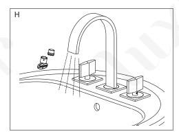
H. Use the aerator wrench to remove the aerator. Turn on both hot and cold handles and let the water run for about 1 minute to flush out any sediment or debris inside the plumbing. Also check for leaks at all connections.
