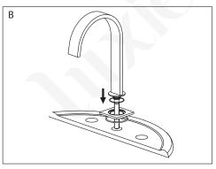
B. Place spout with flange through the center mounting hole on the mounting surface.
