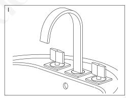
I. Re-install the aerator once all connections are checked. Keep the aerator wrench for future use. The installation is complete at this time.
