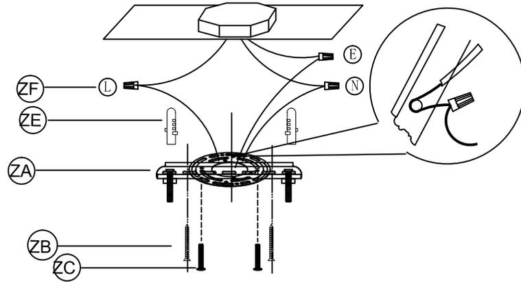
1. Drill two holes on the ceiling and put the plastic anchor screw(ZE) into the holes(If the wall is wood made, this step can be ignored);
