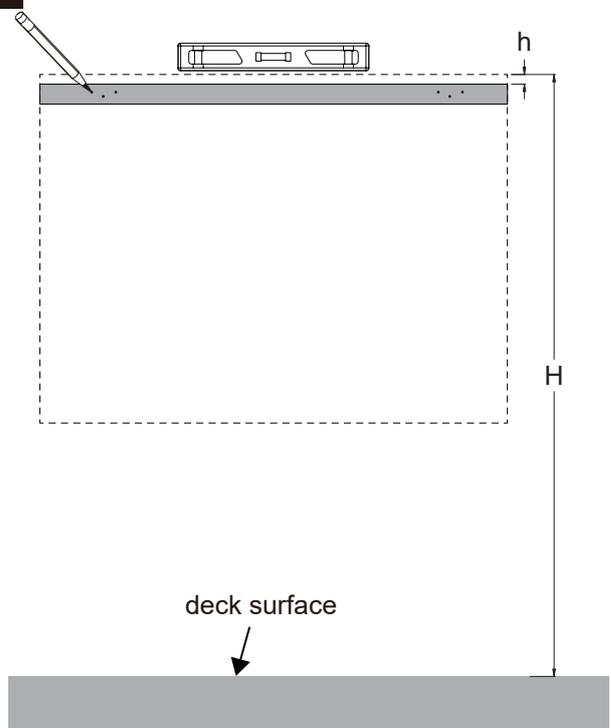
According to the height "H" of the product, place the Position Template horizontally on the wall and mark the installation holes with pencil.
