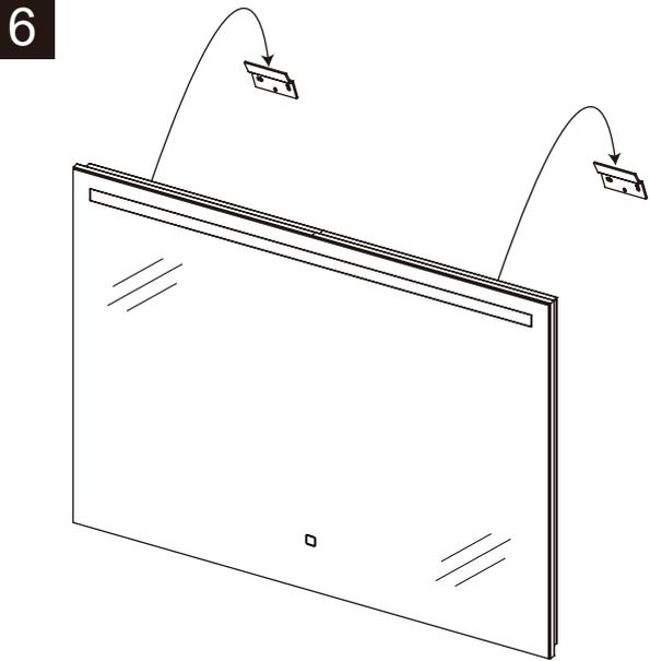
The LED mirror is provided with a power supply cord. For the plug-in connection, hang the mirror to the Hooks as shown. Then plug the power supply cord into the outlet to finish the installation. For the wire connection, please cut the power supply cord near the plug and connect the wire by following step 7. Then secure mirror by following step 6.
