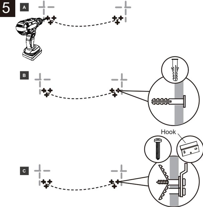
If drilling into wood, drill a 1/8" hole at each marked location (figure A) and secure Hooks with screws. If drilling into concrete, drill a 5/16" hole at each marked location (figure A, B, C), insert wall plugs, and secure Hooks with screws.
