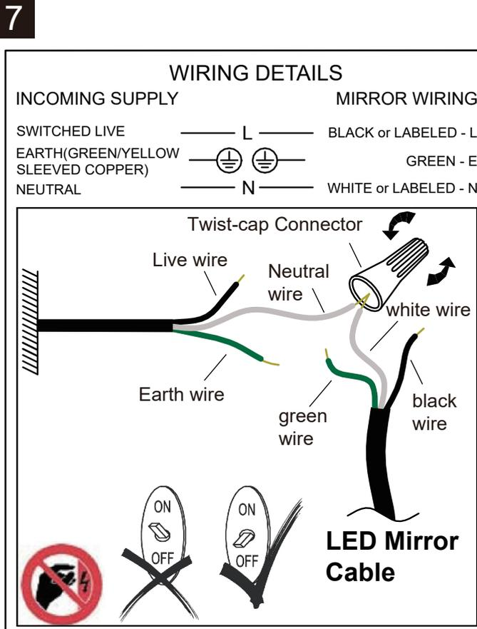
**Before starting the wire connection, please make sure the electricity supply has been turned off.**
