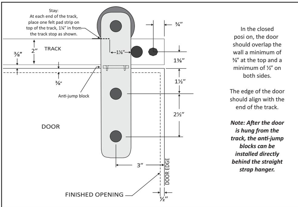
In the closed position, the door should overlap the wall a minimum of 3/8" at the top and a minimum of 1/2" on both sides.
