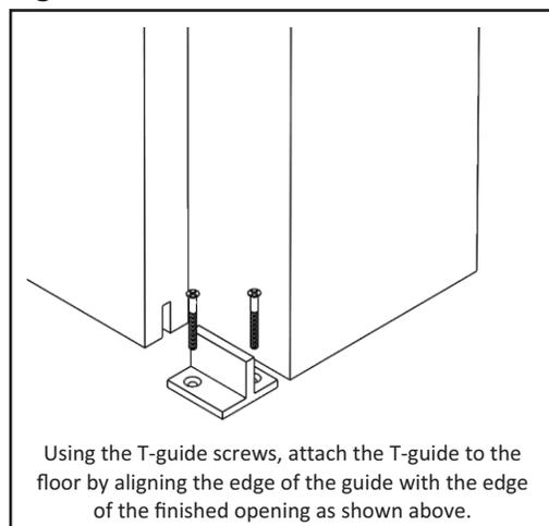
Using the T-guide screws, attach the T-guide to the floor by aligning the edge of the guide with the edge of the finished opening as shown above.
