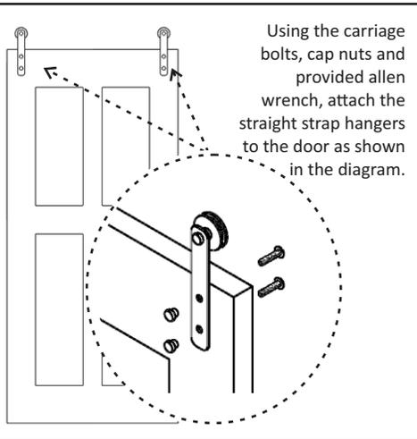
Using the carriage bolts, cap nuts and provided allen wrench, attach the straight strap hangers to the door as shown in the diagram.
