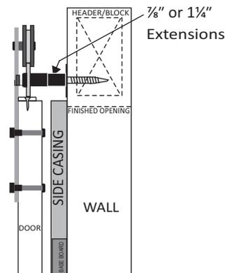
Standard Hardware Pack + 7/8" or 1 1/4" Extension Kit installed where casing, base, or other trim is greater than 1/2".
