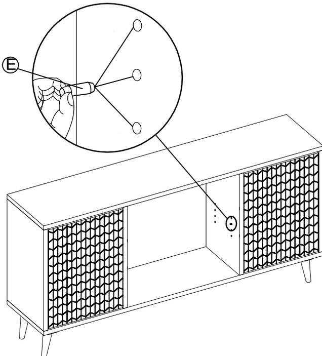
Insert shelf pins into the inner side walls of the cabinet as shown. Carefully place the shelves onto the Shelf pins.
