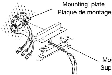
Attach the mounting bracket to the mounting plate with cap nuts provided.
