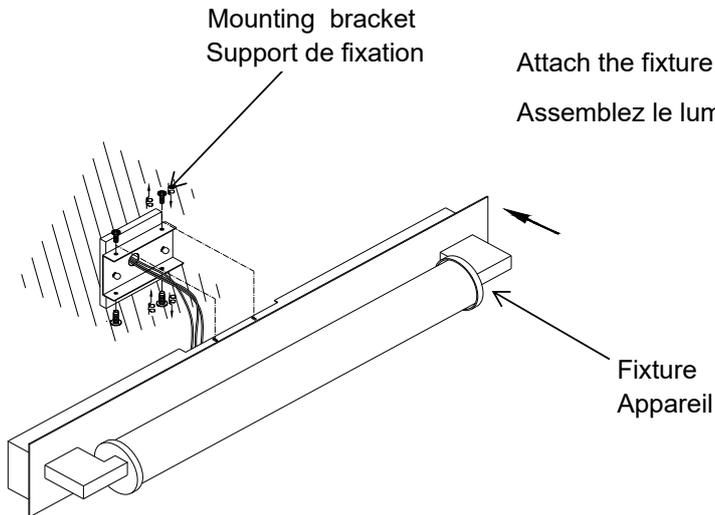
Attach the fixture to the mounting bracket with screws provided.
