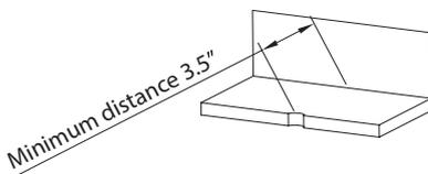
If the distance between the faucet hole and the wall is less than 3.5," position the faucet lever 30° to 90° off the wall to allow for full operation
