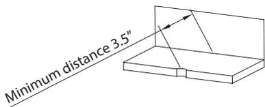
The minimum distance between the faucet hole and the wall should be 3.5"
