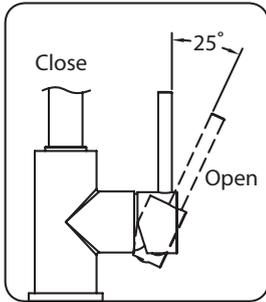
1. Pull the lever to the right to turn on the water. Push to the left to turn off
