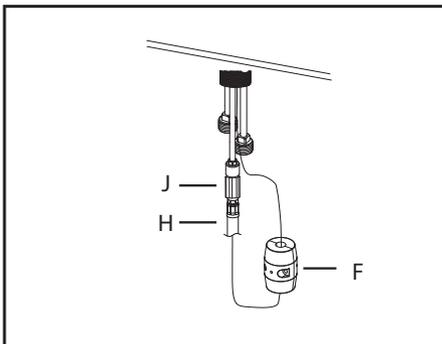
Attach weight (F) to lowest point vertically on spray hose (H)
