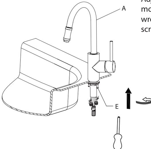
Adjust faucet body (A). Secure mounting hardware (E) with wrench and Phillips head screwdriver
