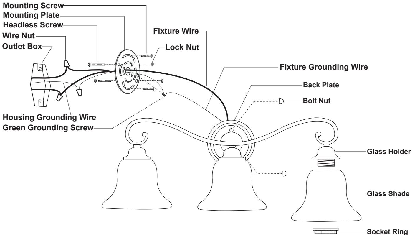
1. Thread two headless screws through the mounting plate, and secure them with four lock nuts (two on each side of the mounting plate). Adjust the length of the headless screws if necessary.
