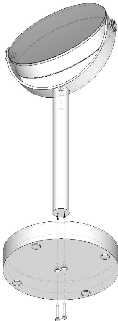
fit the two screws into the base and tighten onto the mirror stem
