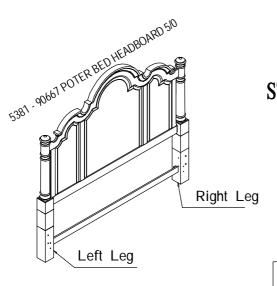
STEP 1: Attach legs to headboard using bolts(A), lock washer(E), flat washer(D), and attach bottom rail to the legs using bolt (B) as shown in step 1. Using an open wrench (G) to tighten all the bolts.
