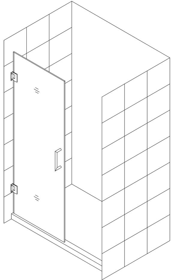
**NOTE:** The Unidoor hinge is factory set to over close 8°. The following procedure is recommended to ensure proper alignment of the panel glass and the door glass.
