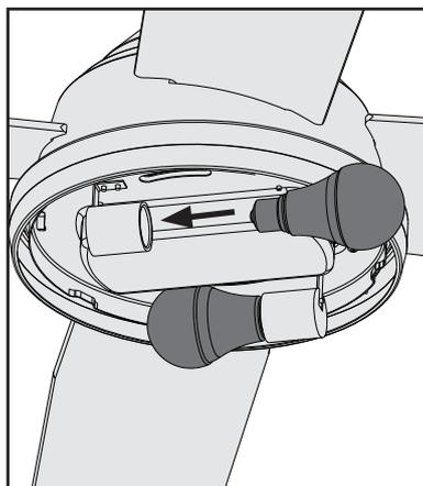
Install a bulb into each of the sockets. When necessary, replace with bulbs of the same type and wattage.
