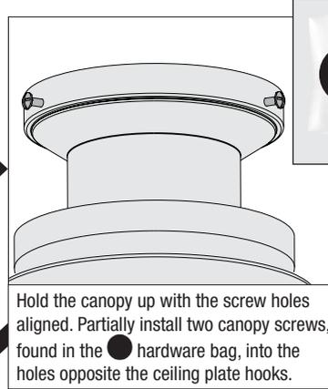
Hold the canopy up with the screw holes aligned. Partially install two canopy screws, found in the ● hardware bag, into the holes opposite the ceiling plate hooks.
