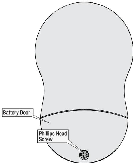
To access the battery compartment, remove the small Phillips head screw that secures the battery door to the transmitter assembly. The battery should be installed with the positive (+) side up. Replace with a CR2032 battery when necessary.
