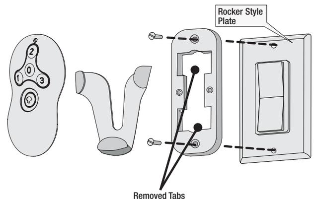
**Note:** For rocker-style cover plates, break off the tabs by pushing outward.
