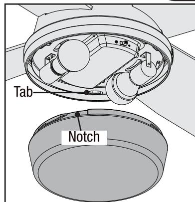
Lift the globe and align the notches in the globe with the tabs in the light kit. Attach the glass bowl to the light kit by twisting it clockwise until it snaps into place.
