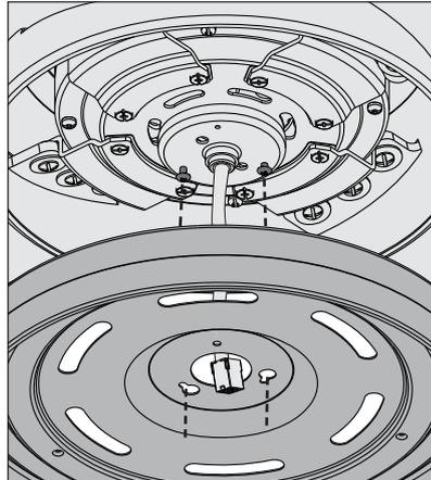
Feed the wire plug through the center hole of the hood, then wrap keyhole slots around the screws and twist counterclockwise.
