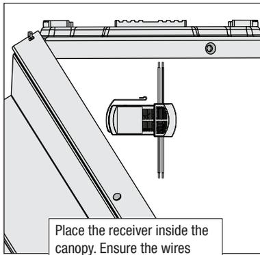
Place the receiver inside the canopy. Ensure the wires remain connected.
