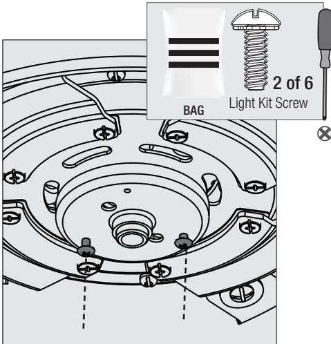
Screw two housing assembly screws from the hardware bag halfway into the motor housing. It does not matter which two screw holes you choose.
