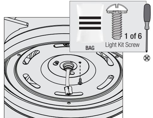
Insert the third screw, found in the hardware bag, into place and then tighten all three screws.
