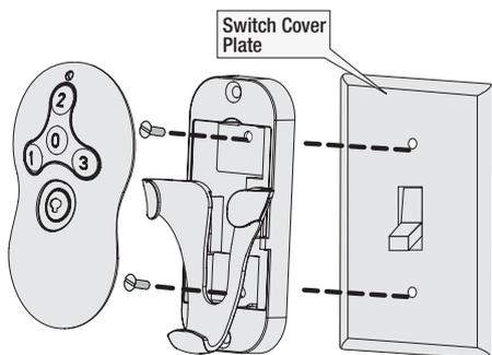
To install the transmitter cradle, remove the two screws holding the switch cover plate. Do not remove the cover plate. Orient the cradle by lining up the two mounting holes with those on the cover plate. Insert and tighten the screws. Do not over tighten.
