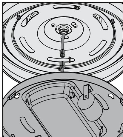
Connect the plugs from the upper and lower switch housings. Make sure to line up the colored markings on the connectors. Wrap light kit keyhole slots around the screws and twist counterclockwise.
