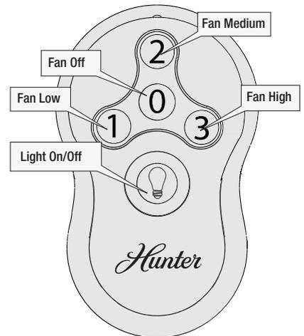
To turn on fan, press a fan speed button. Speeds range from off (0) to high (3). Quickly press the Light button to turn the lights off and on.
