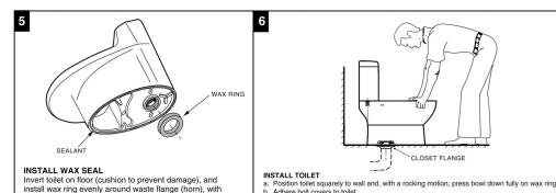
c. Smooth off the bead of sealant around base. Remove excess sealant.
