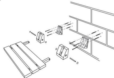
**3. MOUNTING** (Masonry, brick, block wall)
