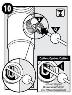
Verify that the white plastic pivot rod seal (S) is in place with beveled side facing out. The pivot rod (Q) can be installed two ways the Illustration shows the pivot rod in the EASY CLEAN position which allows the plug to be pulled out for deaning. The other option (Illustrated in the inset) shows the pivot rod installed in the VANDAL PROOF position. The end of the pivot rod (Q) is inserted into the opening at the bottom of the plug (I).
