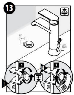
Loosen the pivot rod strap (H) bolt enough to allow the lift rod to move. Position the lift rod knob 5/16" above the faucet and the drain plug 1/2" above the drain seat. Tighten
