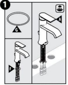
For single hole installations, place deck gasket (F) on the underside of the faucet body (A). Insert faucet into sink opening.
