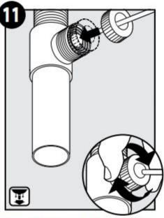
Insert pivot rod into opening and tighten pivot rod nut (P) finger tight.
