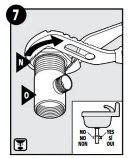
Using an adjustable wrench or channel locks, finish tightening Drain Nut (N). Ensure opening of Drain Body (O) is facing the back of the sink.
