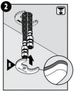
From below the sink, slide the mounting bracket (B) onto the threaded shank.
