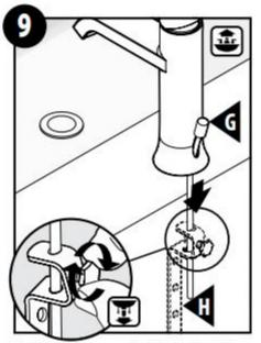
Insert lift rod (G) into open on the back of the faucet body. From below the sink slide the pivot rod strap (H) onto the lift rod (G). Finger tighten the hex bolt head.
