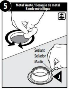
Clean/wipe sink drain area with soft cloth. Apply a bead of sealant to underside of Drain Seat (K).
