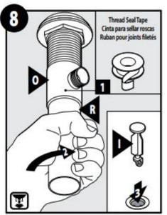
1) Apply thread seal tape to threads on Tail Piece (R). 2) Install Tail Piece (R) to Drain Body (O) and hand tighten.
