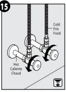
Turn on the water supply line valves on and check for leaks.
