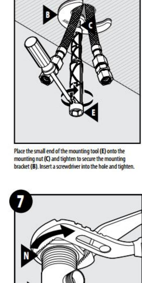
From below the sink, slide the mounting bracket (B) onto the threaded shank.
