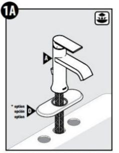
For 3 Hole Applications: Place Escutcheon (D) onto sink and insert faucet body (A) into opening.
