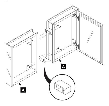
\* Place cabinet (A) on the bottom bracket (K) and secure it with a top bracket (L).
