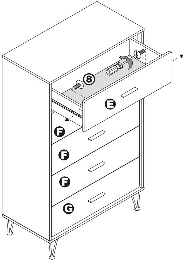
Extend the two outer slides of the runners so that they could align with the sides of the drawer. Make sure the pre-drilled holes from the drawer align with the screw holes of the outer slides. Secure two screws from the inside of the drawer using a Phillips screwdriver to tighten them to the outer slides.
