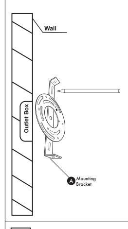
Raise mounting bracket (A) to the wall. Mark location for the plastic anchors (B). Drill holes for plastic anchors (B). Insert plastic anchors (B) into hole.
