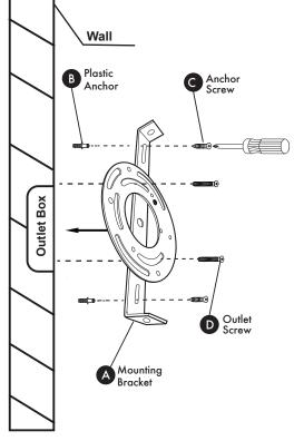
Attach mounting bracket (A) to outlet box with outlet screws (D). Screw anchor screws (C) into plastic anchors (B) to secure mounting bracket (A).
