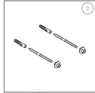
3. Insert the anchors into the drilled holes, screw the mounting hanger bolts.
