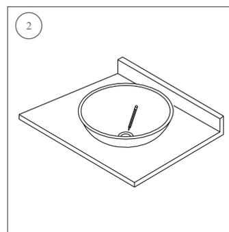
4. Drill a 1 5/8" (41 mm) hole at the marked location. Hole can be larger than 1 5/8" depending on the drain hole size of the specific sink.
