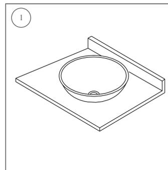
2. Trace the sink drain hole onto the countertop.
