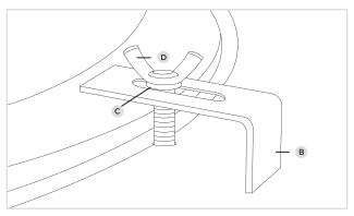
STEP 5 - ATTACH UNDERMOUNT CLIPS
