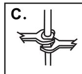
Tighten connection with two wrench to prevent damage to tube body.
