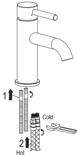
Preparation: Turn off water supplies and drain water lines. Clean installation site and remove any debris from the area.
