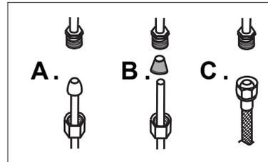
Connect to water supply lines with either:
