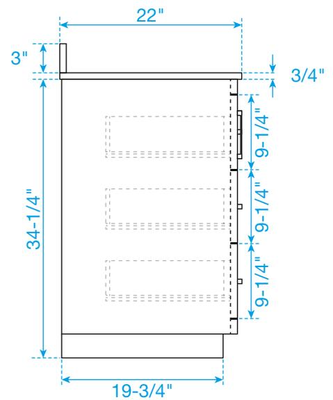
\*Note: Due to high probability of breakage, the backsplash comes in two pieces, cut from the same piece. All measurements are  $\pm 1/4"$ .
