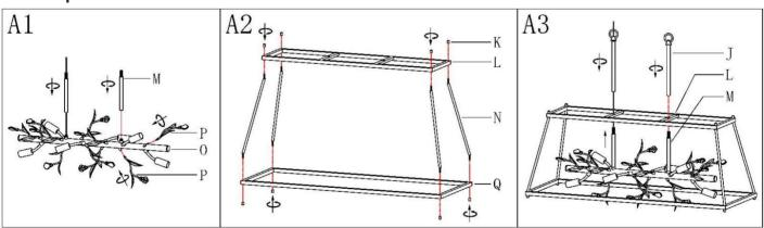
Step A1 » 1) Carefully pass the fixture wires through stems (M), then screw stems (M) onto the top of socket assembly (O).
