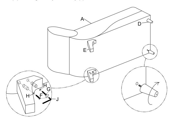
Assembly the Left Arm (B) to the Chaise Body (A) using Bolt (G) and Flat Washer (I), then tighten by Allen Key (J).
