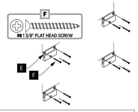
IMPORTANT: Consult an expert for the proper screws/bolts to use when attaching to various constructions. Screws provided do not attach to all wall construction types. Anchors are not required if brackets are installed in stud.
