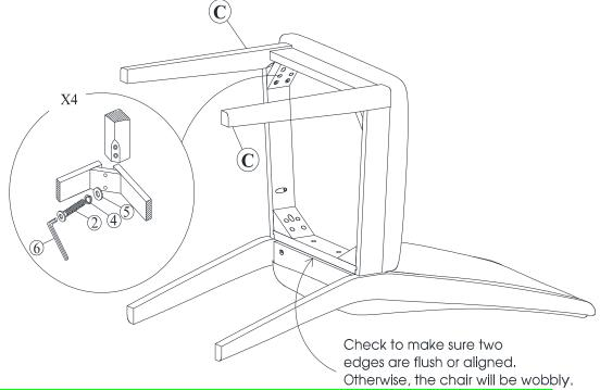
Place the chair on a flat level surface to make sure the chair is levelled and then tighten fully the all bolts.
