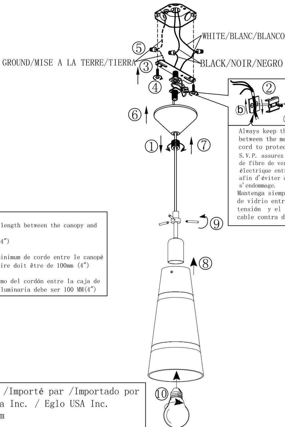
Always keep the fiberglass sleeving between the metal strain relief and the cord to protect the cord from damage
