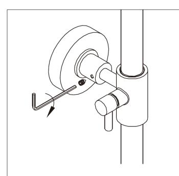
**11.** Slide the shower set into the mounting bracket and secure into place with the set screw.
