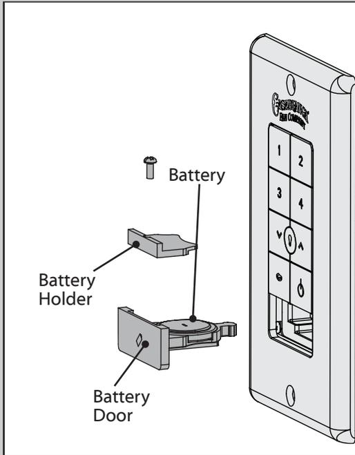
Before operating the wall control, press on the battery door to eject it. Unscrew the battery holder. Insert the battery, found in the control hardware bag, with the positive (+) side facing downward. Reinstall the battery holder and reinsert the battery door into the wall control.
