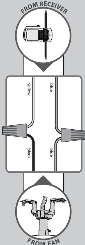
Using the orange wire connectors from the ★ hardware bag:
