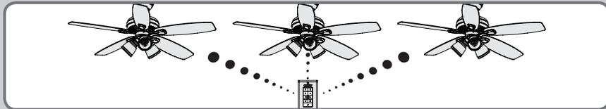
To have multiple fans operated by a single remote control, you must pair the transmitter to each additional receiver. The receiver that shipped with your fan is already paired to the transmitter.
