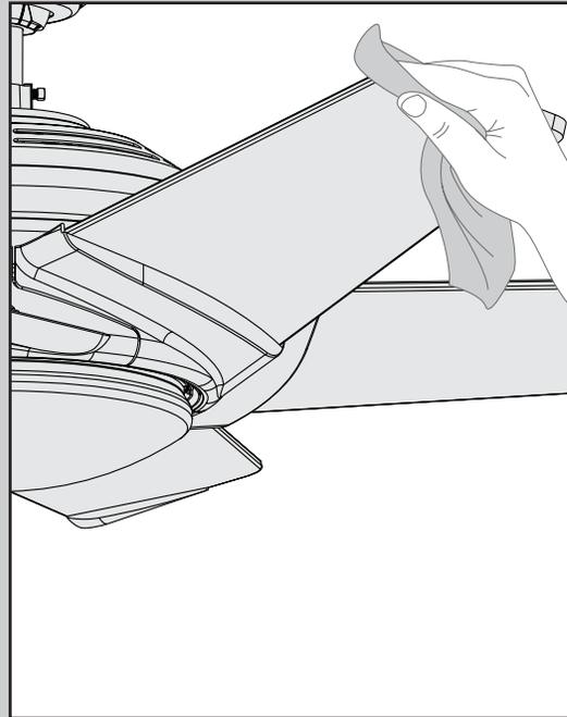
**Cleaning the fan** - use soft brushes or cloths to prevent scratching. Cleaning products may damage the finishes.
