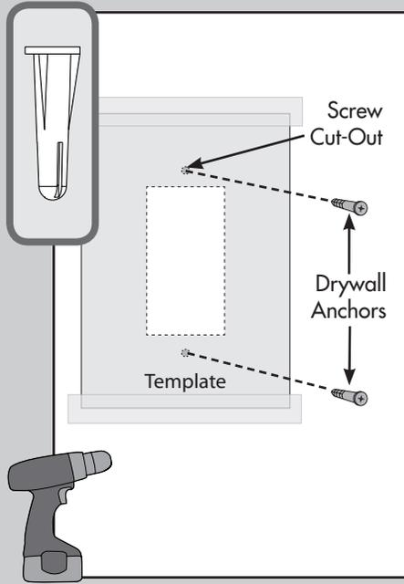
1. Using a 9/64 drill bit, drill a hole in each screw cut-out on the wall control template.
