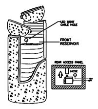
3. FILL RESERVOIR WITH APPROPRIATE AMOUNT OF WATER TO FULLY SUBMERSE THE PUMP.
