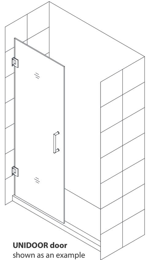
1. Align the **Door** so that it is perpendicular to the wall and parallel with the outside of the threshold. Mark a line on the threshold for reference. Open the door to allow space for the panel installation. (Fig 1)
