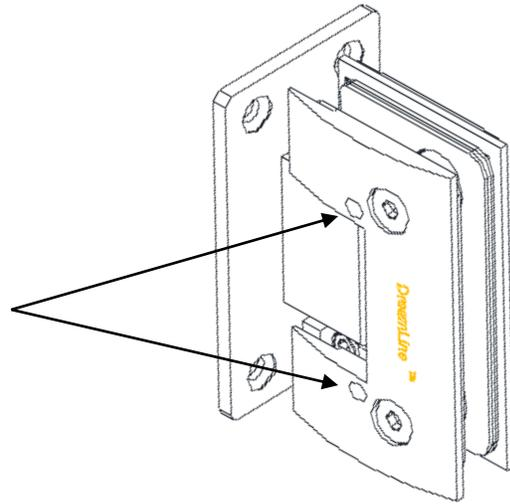
**5a.** Make sure the door glass is plumb and the edge of the hinge is installed flush with the glass edge. Center the hinge in the glass notch and tighten the faceplate screws (**Fig 5a**). Be careful not to scratch the finished surfaces of the hinge during installation.
