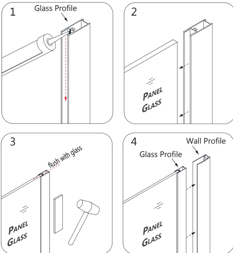
If necessary, use a rubber mallet to tap on the glass profile
