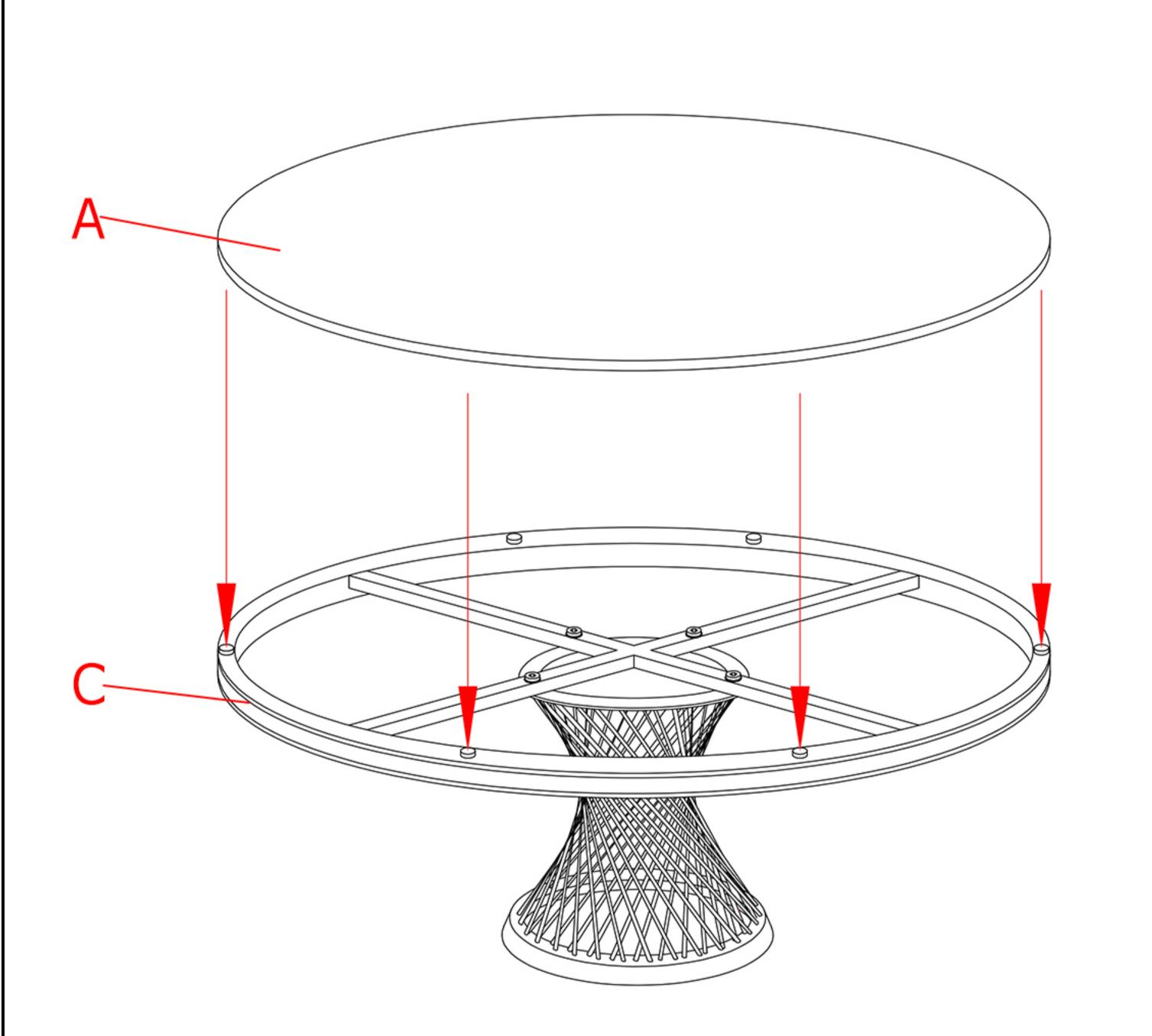
4. Put the tabletop (A) onto the mounting ring (C).
