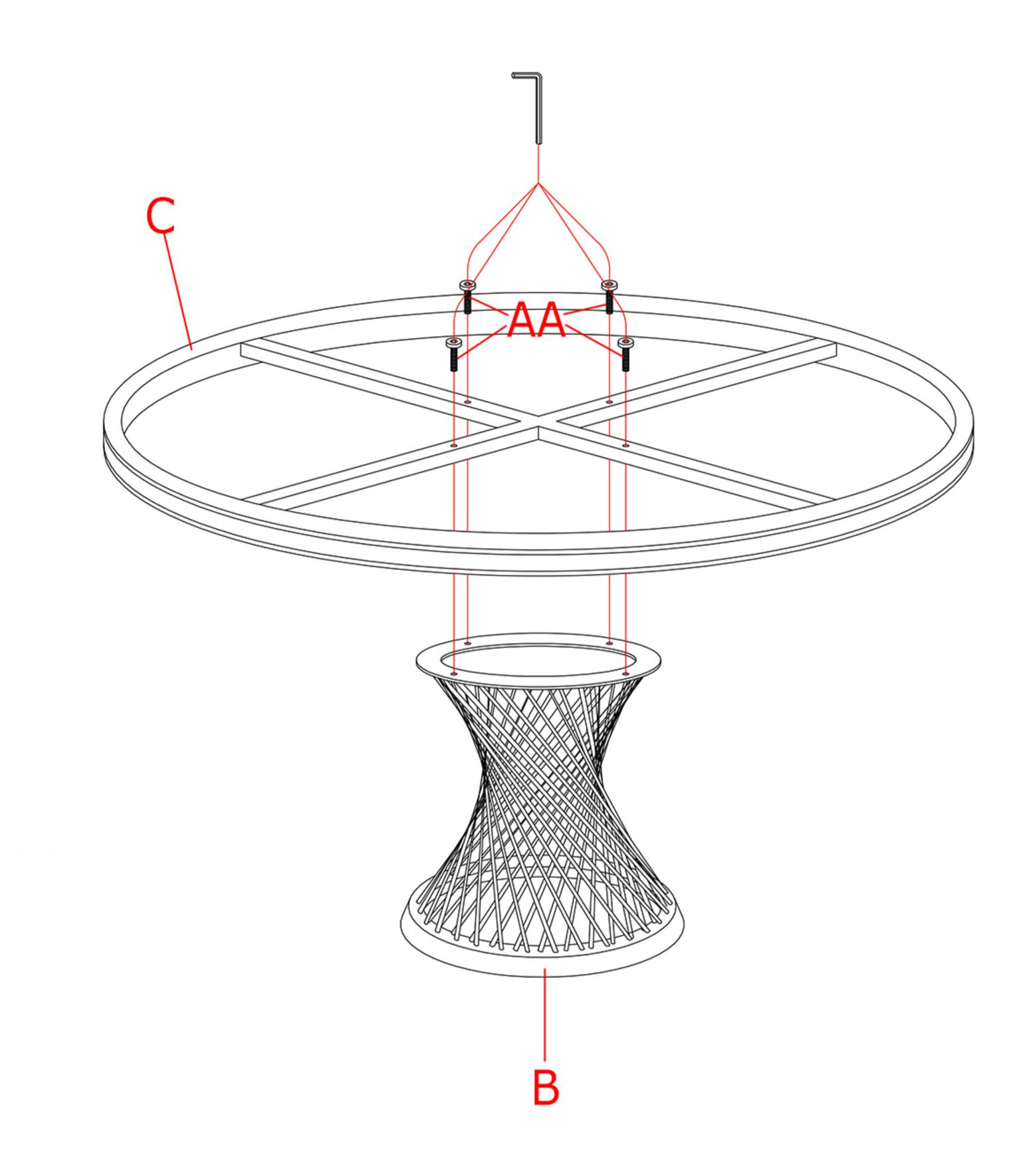
2. Put the mounting ring (C) onto the metal base (B), screw the long screw (AA).
