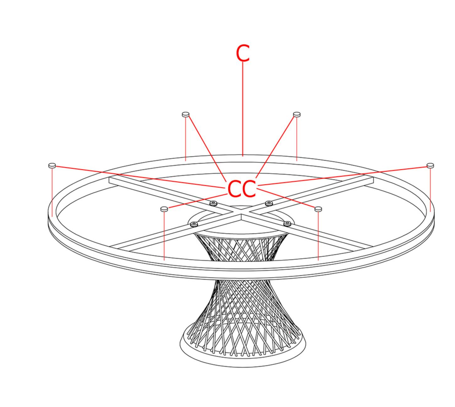
3. Paste protector pad (CC) on the mounting ring (C) as shown.
