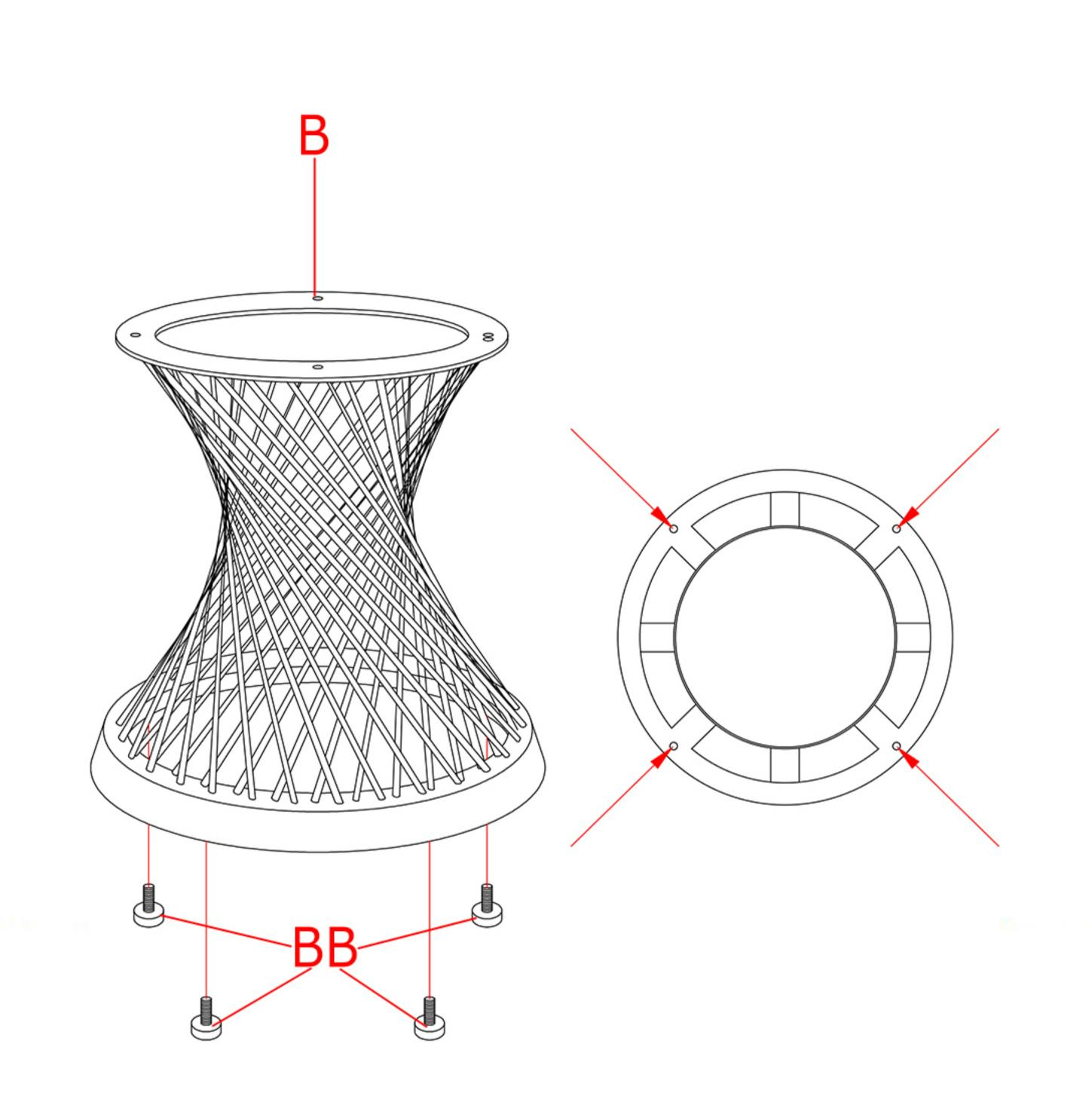
1. Screw the levelers (BB) into the bottom of the metal base (B). Adjust the levelers (BB) to level the metal base (B).
