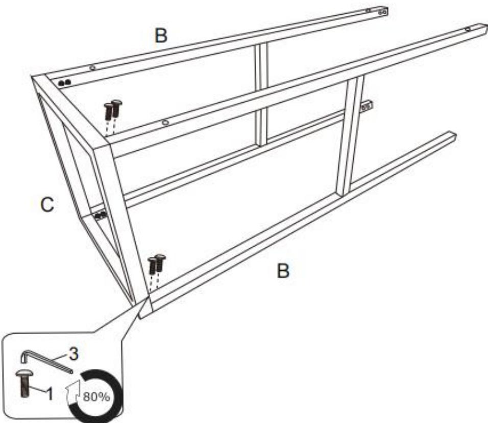
1. Attach the second Leg Connector(B) to second Leg(C) using Allen Key Screws(1).
