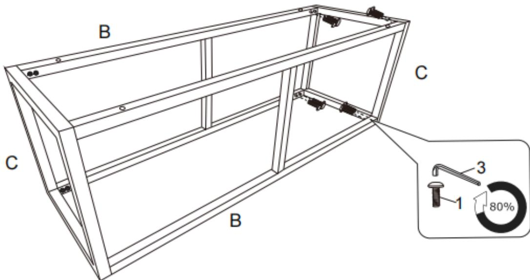
1. Combine both Leg Connectors (B) to both Legs (C) using Allen Key Screws (1).
