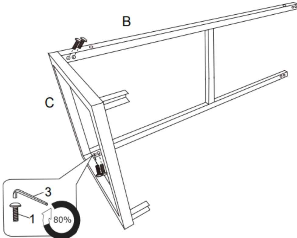
1. Attach one Leg Connector (B) to one Leg (C) using Allen Key Screws (1).
