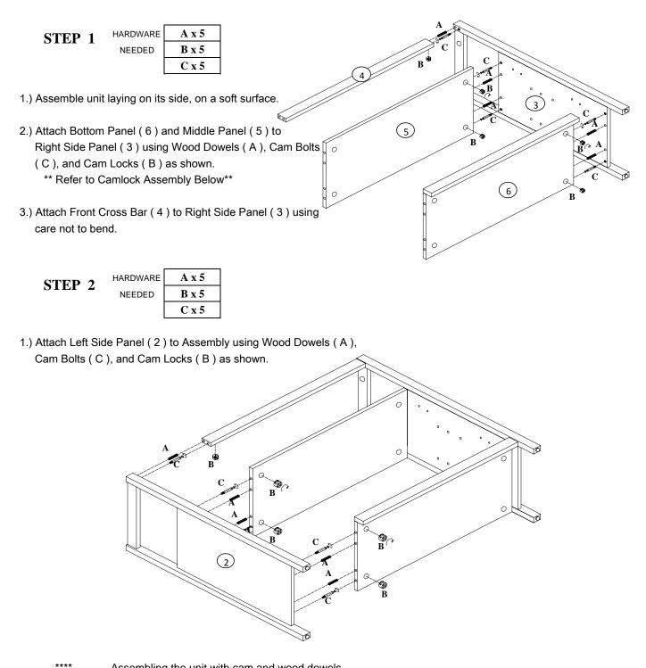
Assembling the unit with cam and wood dowels.
