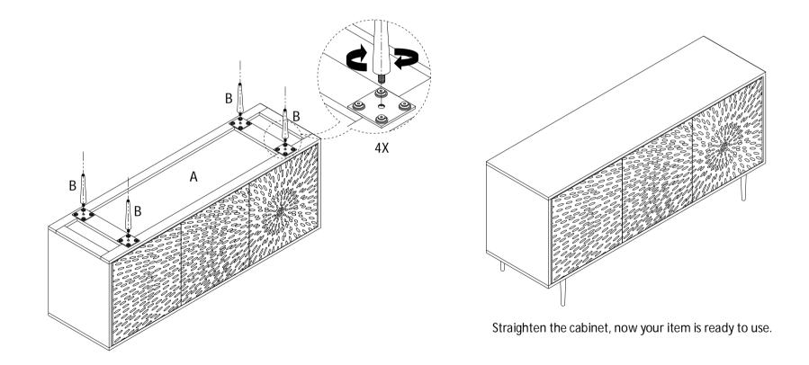
NOTE – Small pin will install in side panel of the cabinet, and large pin will install in mid partition of the cabinet.
