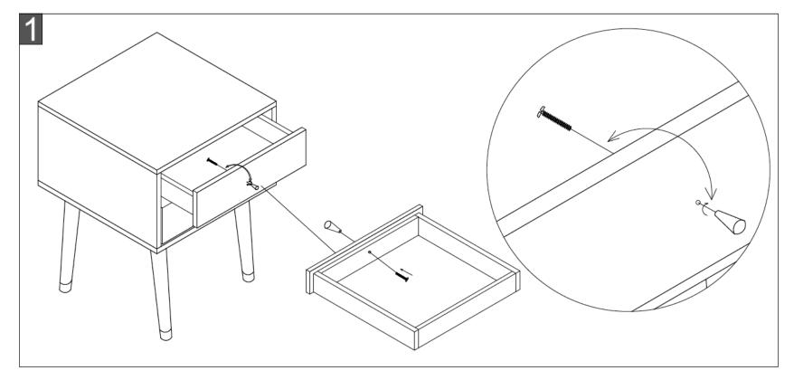
Step 1: Slightly pull the drawer out, assemble the knob to the drawer. Lastly, push the drawer back
