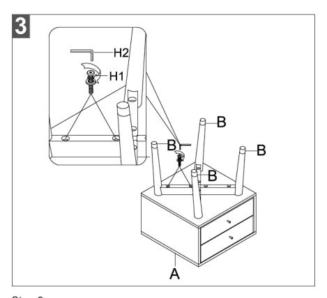
Step 3: Assemble legs (B) with cabinet (A) Use allen key (H2) to lock with 8\*bolts (H1)
