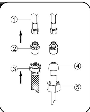
Make connections to water lines with 3/8" female compression supply hoses(1).
