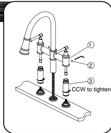
Turn the tubes (3) counterclockwise and reinstall the faucet(1). Tighten the screw (2). Do not overtighten.
