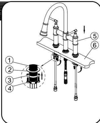
Place new faucet (5) through the three holes in top of sink or countertop (6). From underside, assemble metal washer (2) and nut (3) onto valve body (1) and tighten nut (3). and then tighten the screws (4). Do the same on the opposite side. Do not overtighten.
