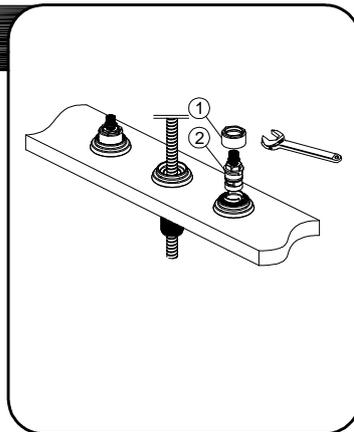
Loosen the cartridge nut (1) and Remove the old cartridge (2) and replace with the new cartridge. Replace the cartridge nut (1) .
