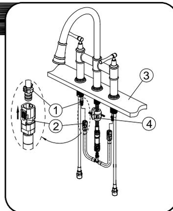
From underneath the sink or countertop (3), align block (1) and tabs (2) on Quick connects. Push Quick connect housing firmly upward and snap onto receiving block. Pull down moderately to ensure connection has been made. If it is necessary to remove quick connect, squeeze tabs on hose between index finger and thumb, then pull down to disconnect. After connecting the hose, install the weight (4) at the lowest point of the hose.
