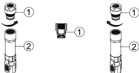
The faucet ships with a 1.5GPM aerator installed. An optional 2.2 GPM aerator is also included in the box. To switch the flow rate of the faucet:
