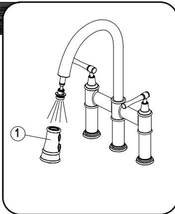
To prevent damage to the internal parts of your faucet from debris that may have collected in the water lines, it will be necessary to flush the faucet. Remove spray head (1). Turn on hot and cold water supplies. Flush water lines for one minute. Reinstall the spray head tightly.
