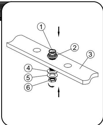
Shut off water supplies. Clean sink or countertop surface. Place flange assembly (2) through the center hole on the sink or countertop (3). Then lock it with rubber washer (4) and metal washer (5) and nut (6). Then place the rubber washer (1) on the flange.
