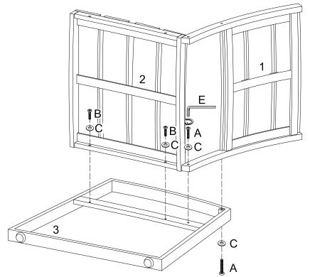
Use washer (C), bolt (A)(B) and wrench (E) to assemble the side frame (3) to the seating panel (1)(2) as shown as diagram.
