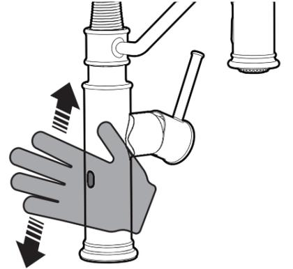
**NOTE: SENSOR FAUCET WILL ONLY OPERATE WITH THE HANDLE IN THE "OPEN" POSITION.**
