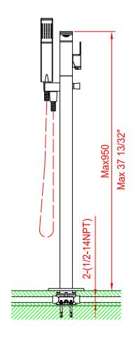
Then drill 4 holes with size Ø8 on the marking places, then put the expansion plugs(7) into the holes respectively.
